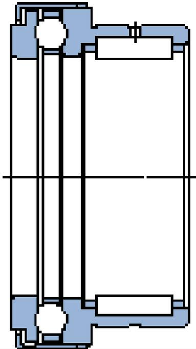
**NKX 70 Z SKF Nadel-Axial-Rillenkugellager NKX..Z**
