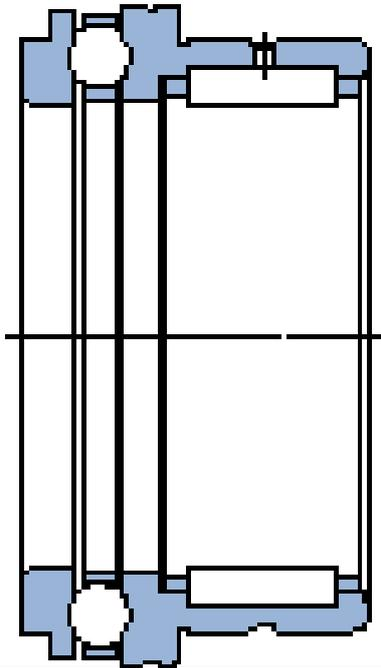
**NKX 10 TN SKF Nadel-Axial-Rillenkugellager NKX..**
