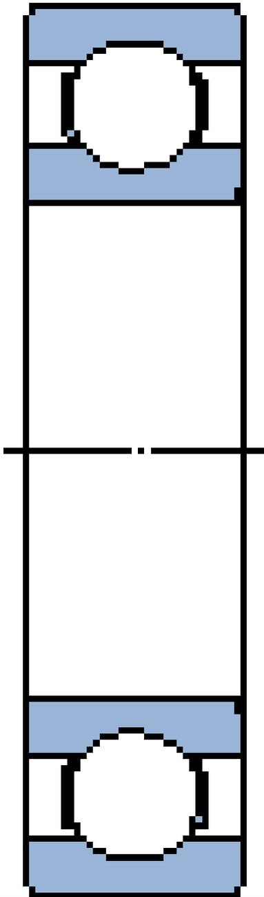
**6204 MA/C3 SKF Rillenkugellager, einreihig**
